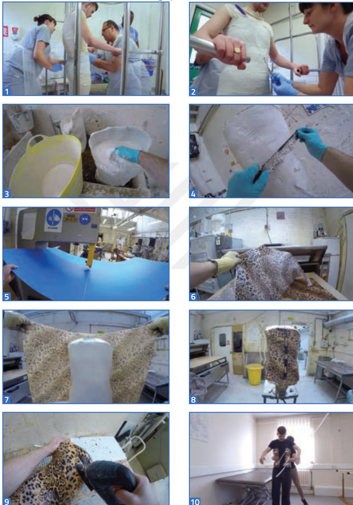
Figure 14 Traditional method of brace making process
