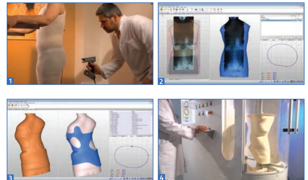
Figure 15 CAD/CAM method of brace making process
