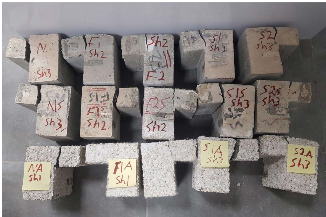
Figure 4.12 Variation in shear strength polypropylene reinforced self-compacting concrete with different environment and fiber fraction volume.
