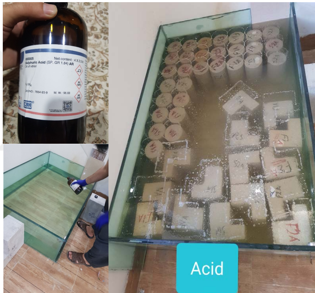
Figure 3.16 details of specimen's exposure to H_2SO_4 .
