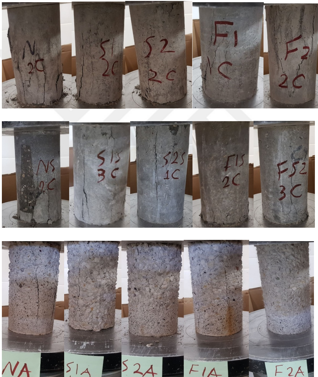
Figure 4.7 Failure modes of FRSCC cylinder samples after compressive test.
