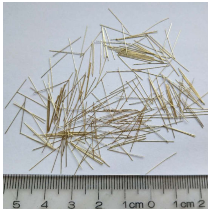
Figure 2.2 Copper coated straight steel fibers.
