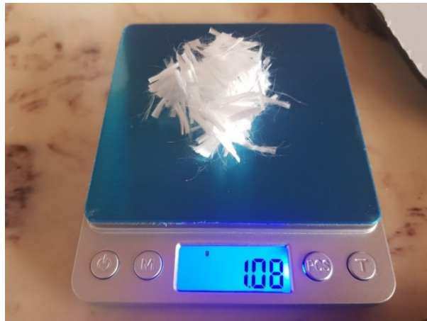
Figure 2.11 Polypropylene fiber used in this research
