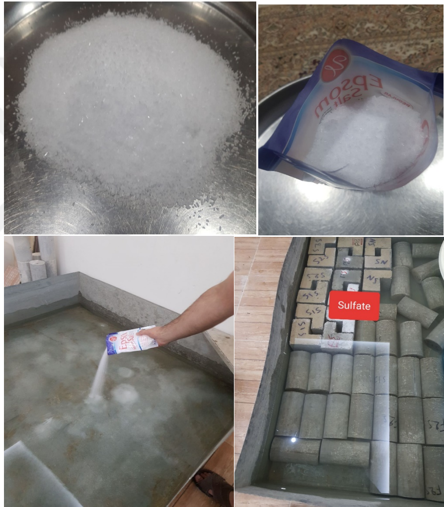
Figure 3.13 details of specimen's exposure to \text{MgSO}_4
