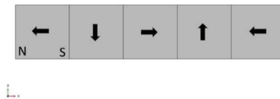
Figure 11. 2D view of the Halbach array design consisting of five neodymium magnets.
