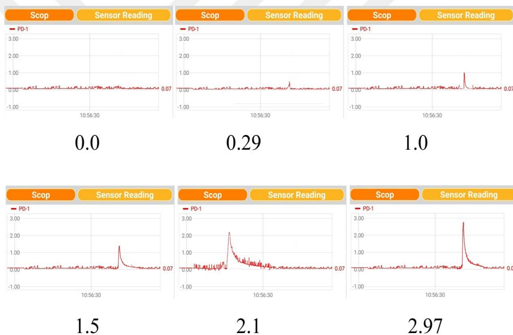
Figure 4.163 The measurement signals for the calibration graph of \text{Fe}^{3+}
