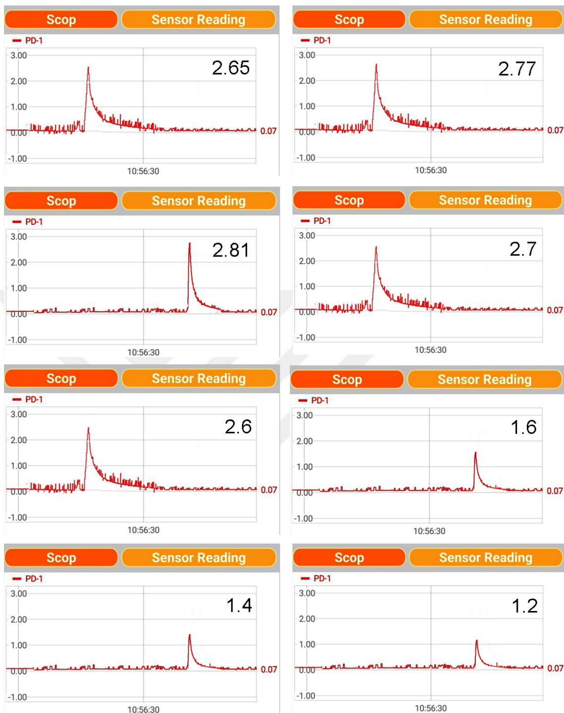
Figure 4.9 The measurement signals obtained against the increased concentration of hydrogen peroxide
