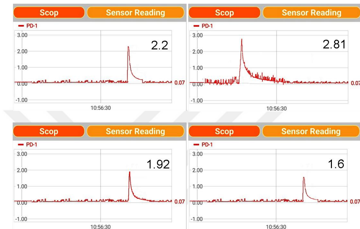
Figure 4.7 The measurement signals obtained against the volume of increased hydrogen peroxide
