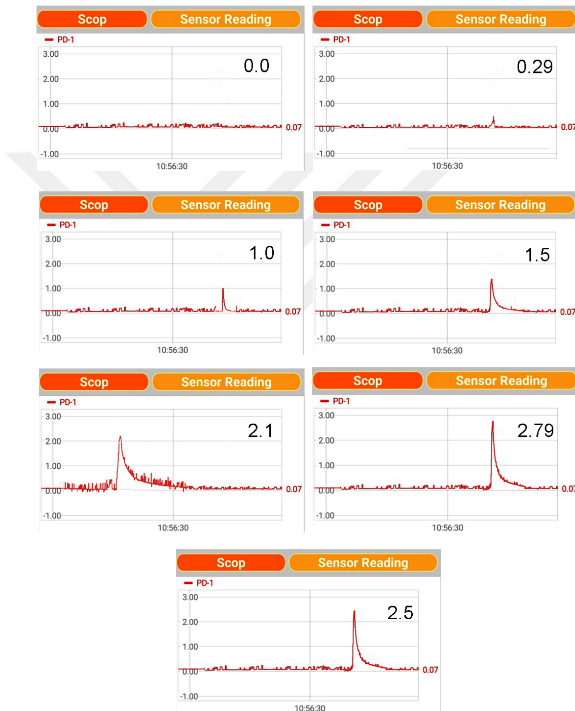
Figure 4.11 The variations in signal intensity with ferric ion concentration
