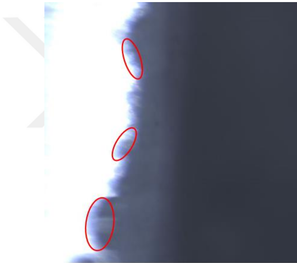
Figure 5.56. Mushy zone and dendrite lengths of RT-62 HC PCM.
