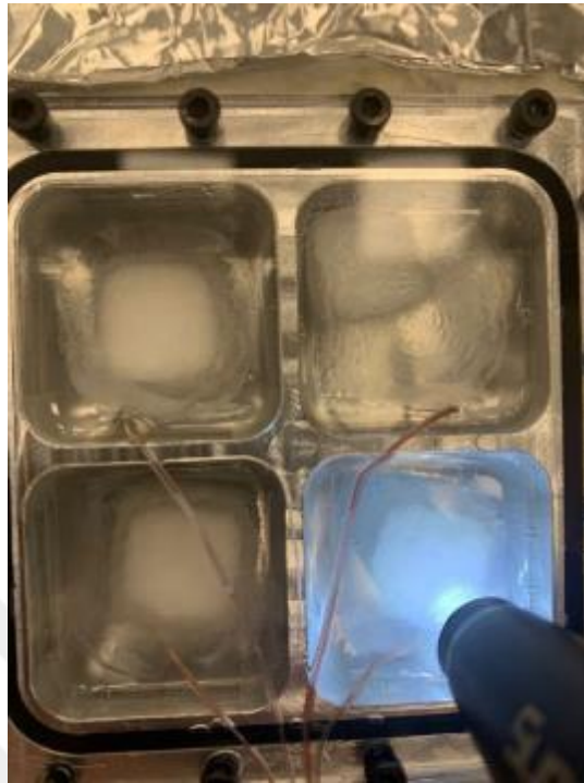
Figure 5.14. 4 Chamber PCM heatsink contours for 0^\circ inclination angle at the 30 th minute with A58H PCM.
