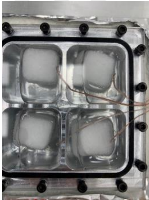
Figure 5.15. 4-chamber PCM heatsink contours for 15^\circ inclination angle at the 30 th minute with A58H PCM.
