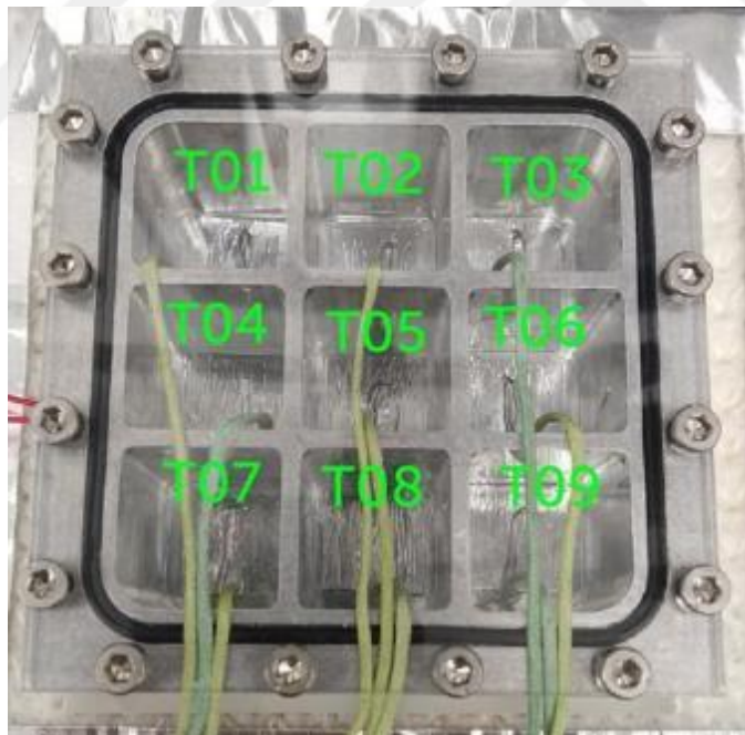
Figure 3.19. Thermocouple positions for 9 chambers heatsink.
