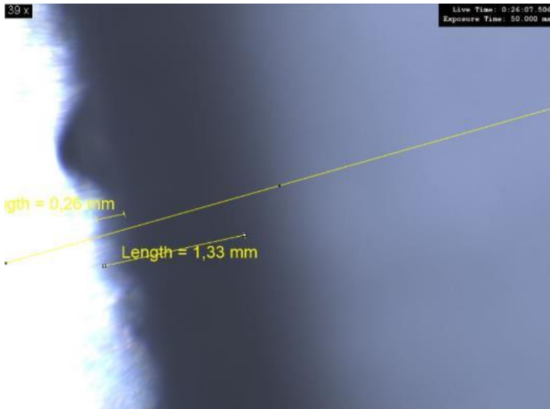
Figure 5.58. Mushy zone and dendrite lengths of RT-70 HC PCM.
