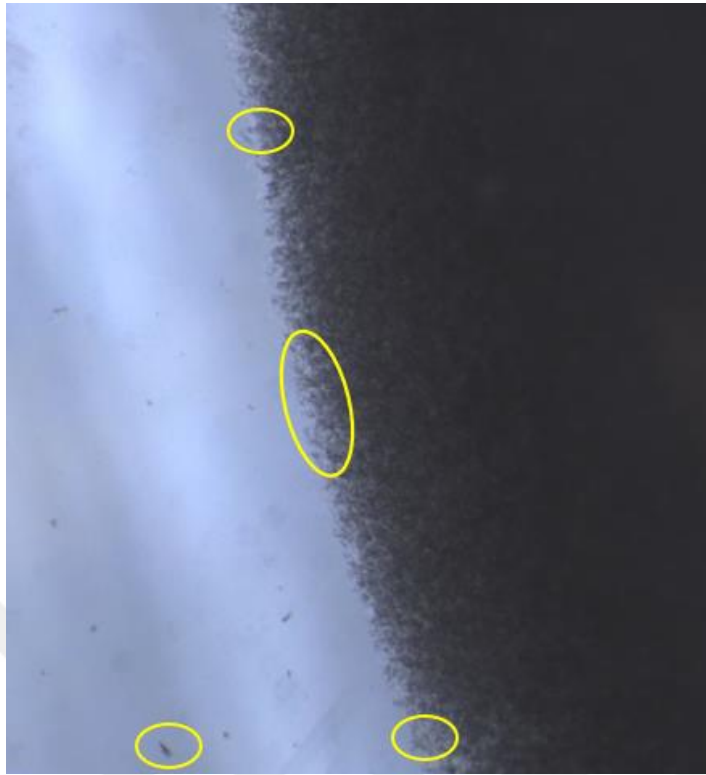
Figure 5.55. Mushy zone and dendrite lengths of A58H PCM.
