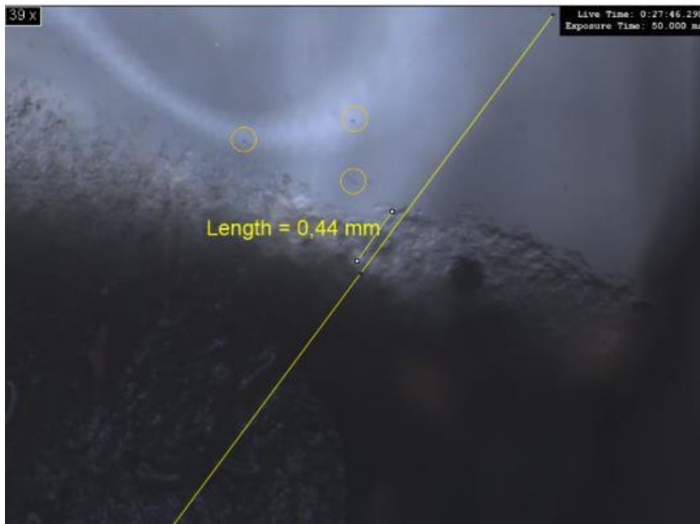
Figure 5.59. Mushy zone and dendrite lengths of A70 PCM.
