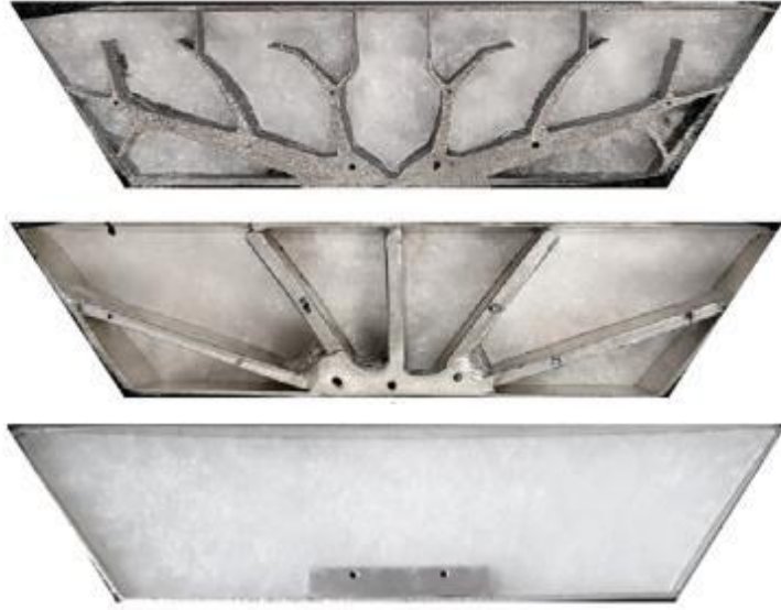
Figure 2.19. Investigated types of heatsinks in the study of See et al. [66] (From top to bottom; topology optimized heatsink, finned heat sink, benchmark heatsink.)
