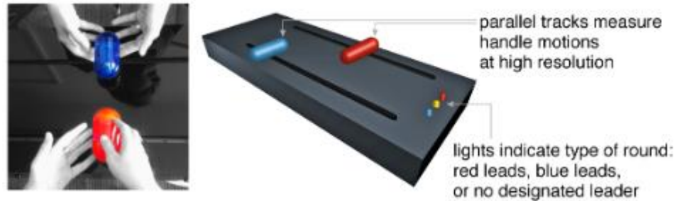
Fig. 2.3. Experimental setup for MG [22]
