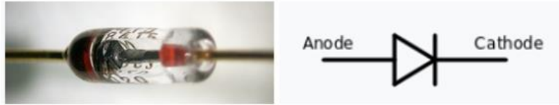
Figure 2.26 : (a) Diode, (b) Diode symbol.
