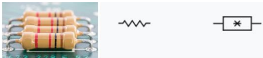
Figure 2.22 : (a) Resistor. (b) Resistor symbol.
