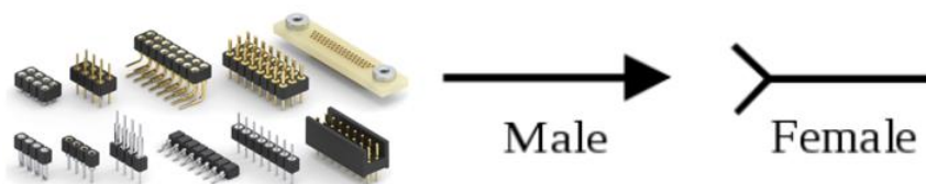
Figure 2.28 : (a) Connector. (b) Connector symbol.
