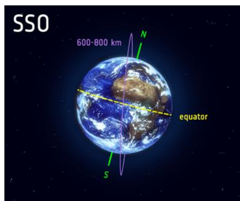
Figure 2.5 : Polar orbit and sun-synchronous orbit (SSO).
