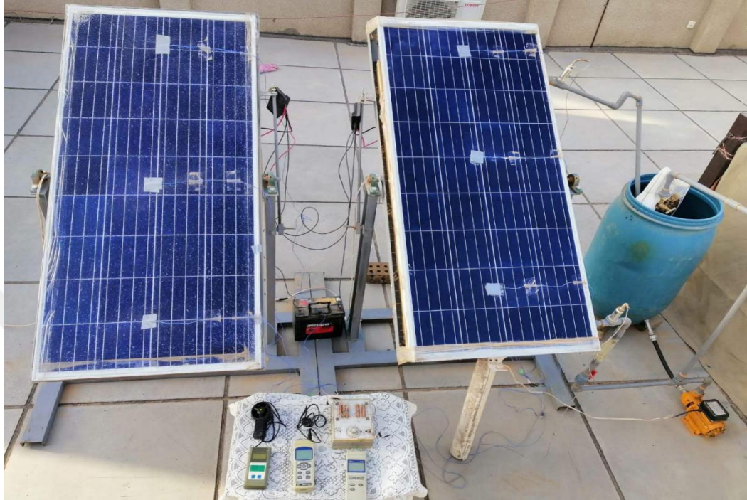
Figure 4.8. Experimental setup of the PV and PV/T system.
