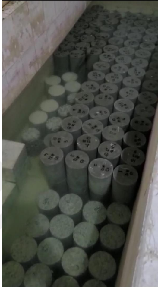
Figure 4.7 Curing Specimens in the Water Storage Tank
