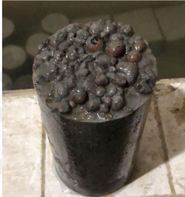
Figure 4.11 Segregation in Mix #3
