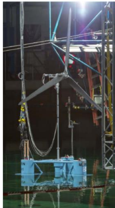
Figure 2.3: OC5-DeepCwind model in the MARIN offshore basin (Source: Helder and Pietersma, 2013)
