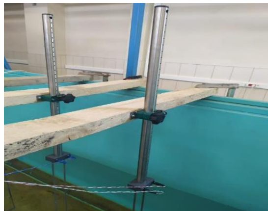
Figure 3.15: Wave gauges installation in the wave channel (Source: Özkol et al., 2022)
