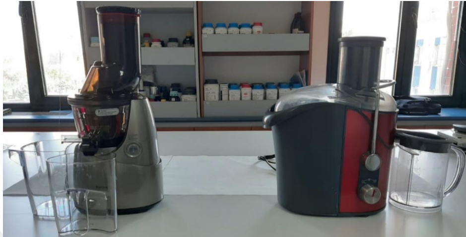
Figure 2.1. Cold-Press juice extractor and centrifugal juicer
