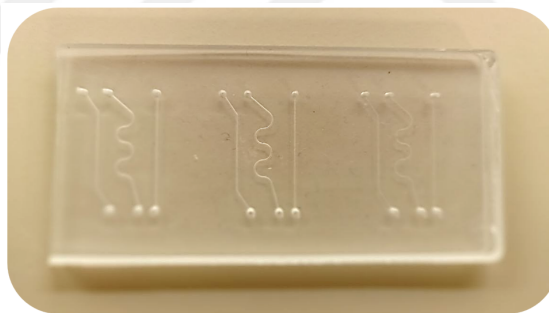
Figure 3.10 Fabricated PDMS chip
