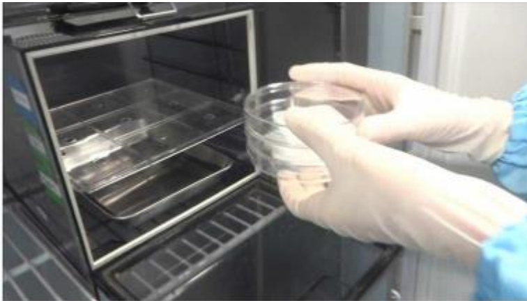
Şekil 3.3. Numunenin inkübasyon aşaması (ISO 22196 Measurement of antibacterial activity on plastics and nonporous surfaces Tadashi Tsuchiya Japan Food Research Laboratories).
