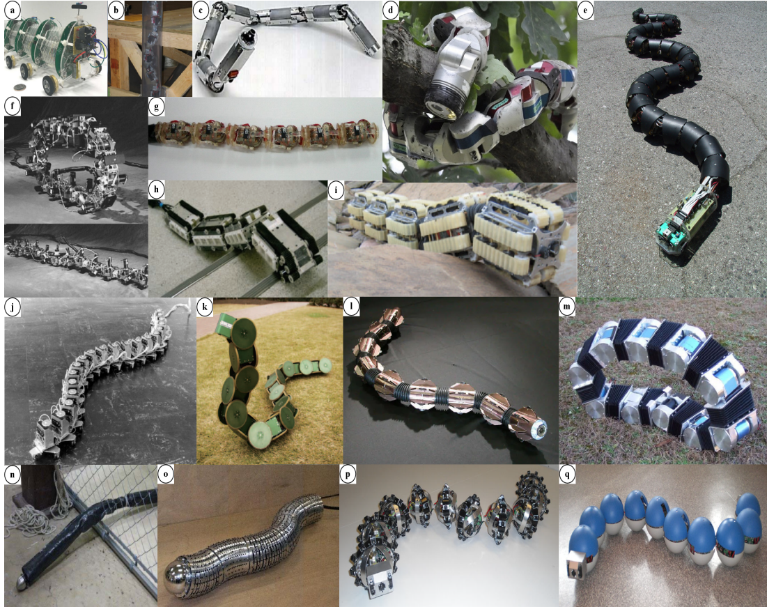
Figure 1.1: Snake robot examples with distinct architectures and capabilities. (a) OriSnake Origami Inspired Snake Robot [1], (b) Modular Snake Robot Climbing the Inside of a Pipe [2], (c) USAR-ETR Urban Search and Rescue Elephant-Trunk Like Snake Robot [3], (d) Unified Snake Robot [4], (e) S5 Snake Robot [5], (f) PolyBot Self-Reconfigurable Snake Robot [6] [7], (g) Pipe Inspection Modular Micro Snake Robot [8], (h) MOIRA2 Inspection Snake Robot [9], (i) OmniTread OT-4 Serpentine Robot [10], (j) ACM III [11], (k) ACM-R3 [12], (l) ACM-R5 Amphibious Snake Robot [13], (m) ACM-R7 Loop Forming Snake Robot [14], (n) Snake Robot with Toroidal Skin Drive [15], (o) Slim Slime Robot (SSR) Flexibly Deformable Snake Robot [16], (p) Wheeko Snake Robot [17], (q) Kulko Snake Robot for Uneven and Cluttered Environments [17].
