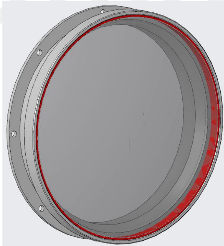
Figure 3.9. CAD model of the front lens and its holder
