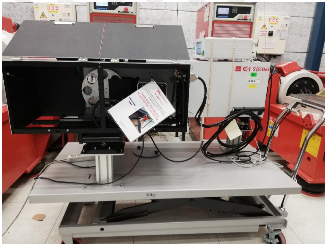
Figure 5.3. Open cover of the collimator showing the target wheel
