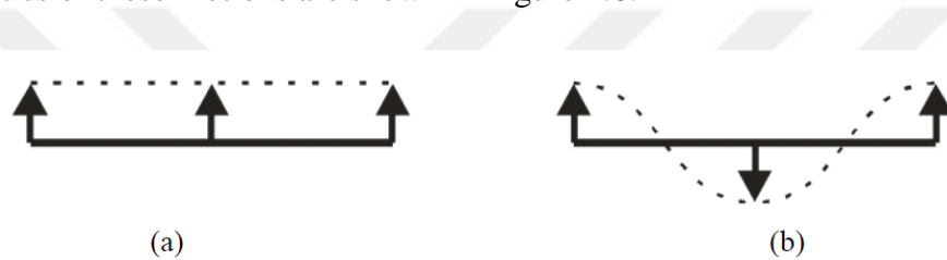
Figure 1.6. Rigid-body motion (a) and elastic deformation (b) on the surface of an optical component under random vibration [3].
