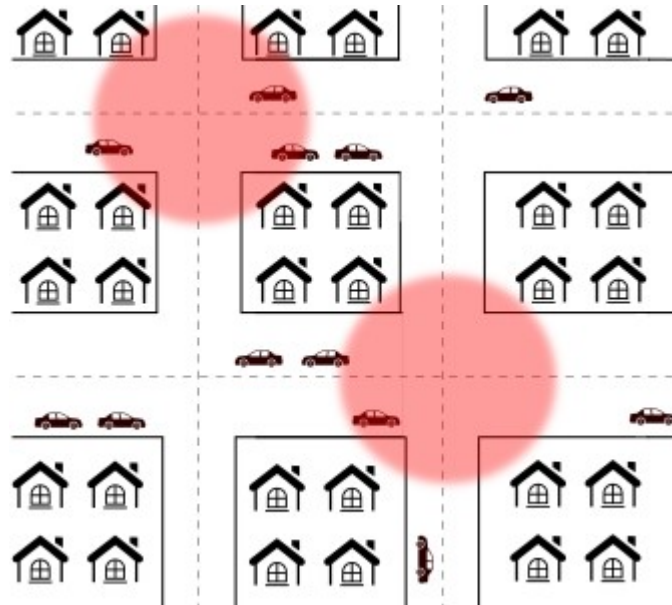
Figure 2.1. Two example observer points in an urban area, which can collect broadcasted CAM messages under the highlighted red range.
