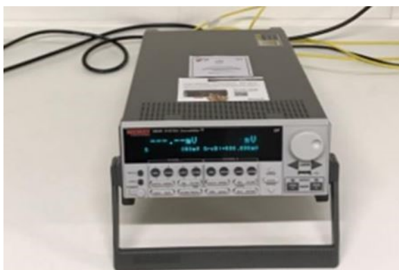
Figure 3.3 – A source meter used to record I – t and I – V measurements.
