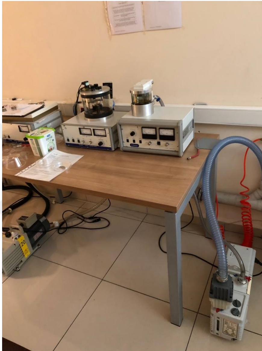
Figure 2.1: A typical PVD for carbon and gold coating in nano-manufacturing.
