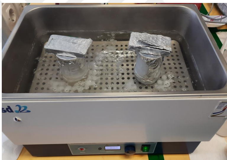
Figure 4.19. A and B phases placed in a digital water bath at 80 °C
