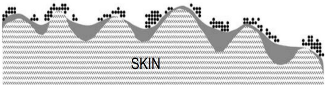
Figure 3.8. Discontinuous coverage resulting water phase evaporation [108]
