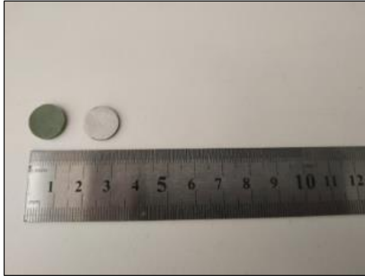
Figure 3.2: The picture of uncoated and silver electrode coated bulk ceramics.
