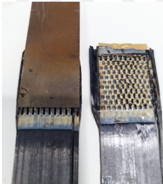
Figure 5.9 Shear-out and pull-out failures
