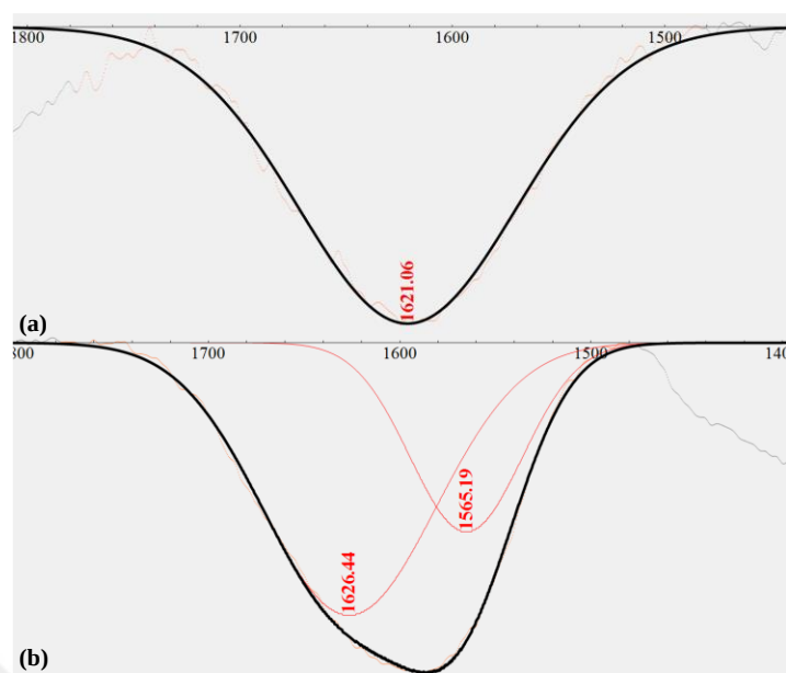
Figure D.2. Deconvolution of ATR-FTIR spectra in the wavenumber range of 1750-1500 \text{cm}^{-1} for (a) Sample 170 °C 9 h. (b) Sample H.
