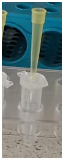
Figure 3.1. A microcentrifuge tube with a HILIC stage tip.
