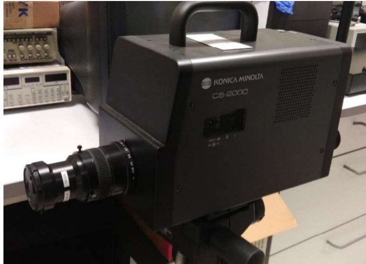
Figure 3.10: Photograph of our used radiospectrometer for brightness measurements.
