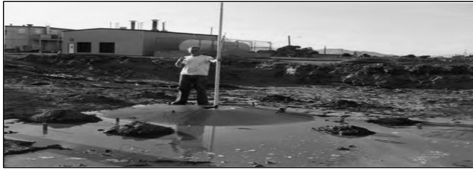
Figure 1.11: The sand boils that caused by the discharge of the excess pore water pressures through the explosive compaction or blasting method [1].
