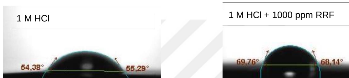
Figure 4.6. Contact angles of Cu surface after exposing to 1 M HCl solution in the absence and presence of 1000 ppm RRflower
