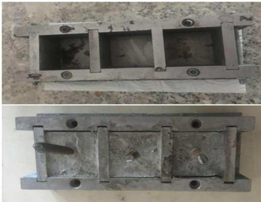
Figure 3.2. 4 x 4 x 16 cm prismatic specimens
