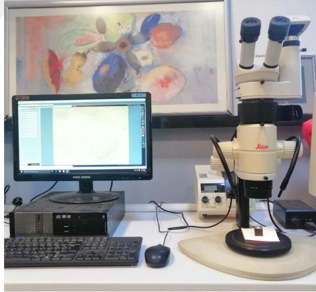
Resim 27: Leica MZ 7,5 stereomicroscope; Leica Microsystems, Almanya
