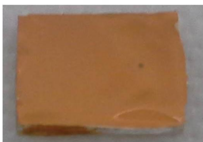
Figure 43. Image of a successfully stripped gold film by thermal curing of SU-8.
