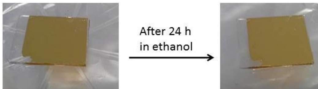
Figure 45. Successfully stripped gold by UV-Visible assisted cross linking.
