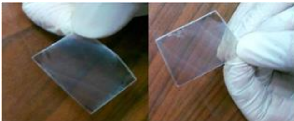
Figure 77. Contamination observed on mica substrate upon heating.
