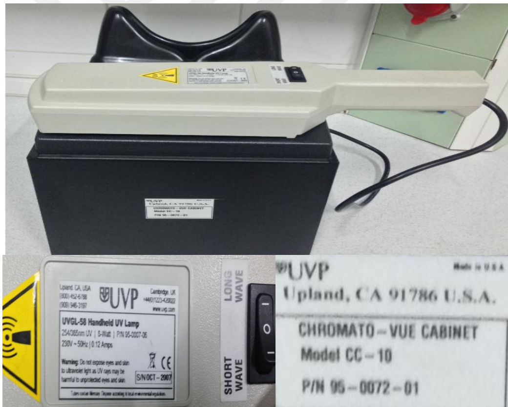
Figure 2.2 The UV-radiation source and the cabinet used in the application
