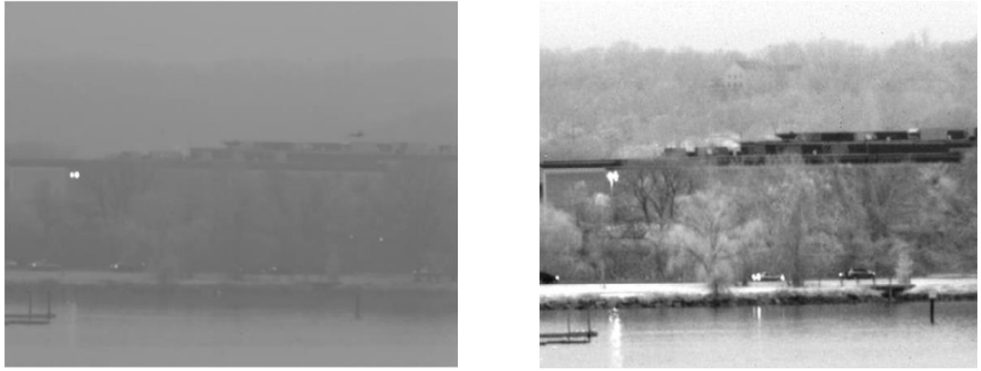
Figure 2.1: Images recorded under hazy conditions by a visible camera (left) and a SWIR camera (right) [12].
