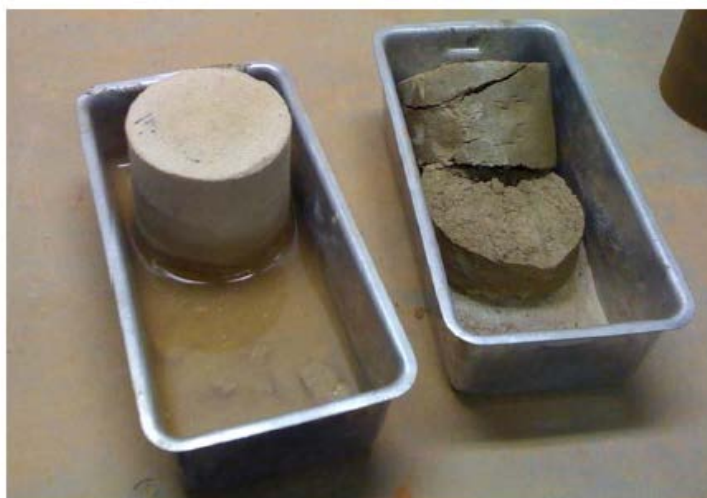
Figure 2.28 : Maintain friction value of CBR after getting soaked (Zydex Industries Ltd.).
