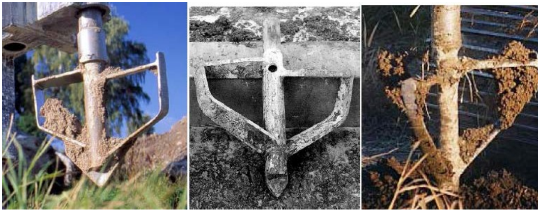
Figure 2.13 : Three versions of the Nordic dry mixing —standard tool (Larsson, 2005).
