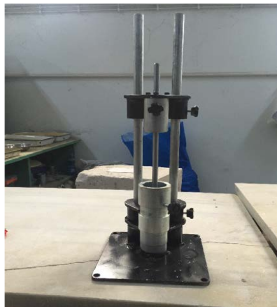
Figure 3.1 : Harvard Miniature Compaction Apparatus.
