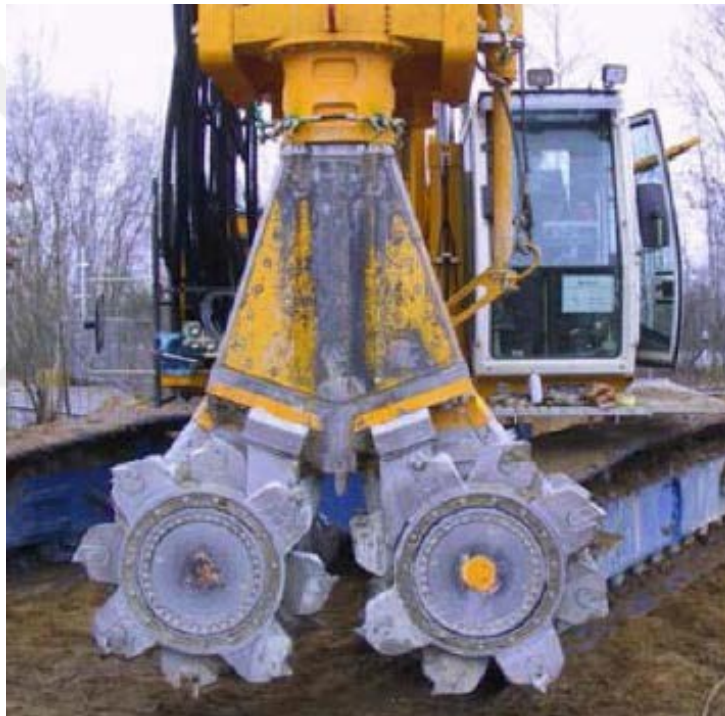
Figure 2.17 : Bauer cutter soil mixing. (Fiorotto et al, 2005).
