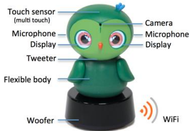
Figure 17 Components of Ixi (Dirkx & Van de Aalst 2014)
