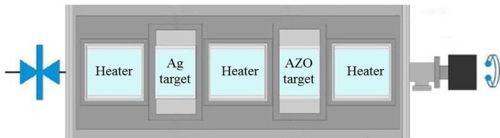
Figure 37: Schematic view of the sputtering chamber
