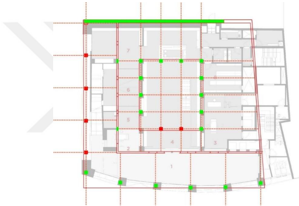
Figure 3.7. The superimposition of the old Yapı Kredi Bank's and YKKS building's structures.
