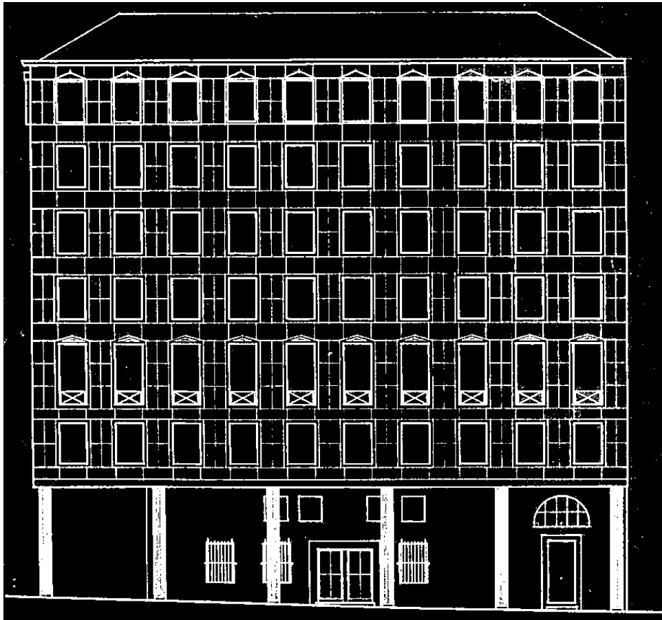
Figure 2.29. Drawing inverted to highlight the order or the Travertine plates on the façade of the old Yapı Kredi Building.
