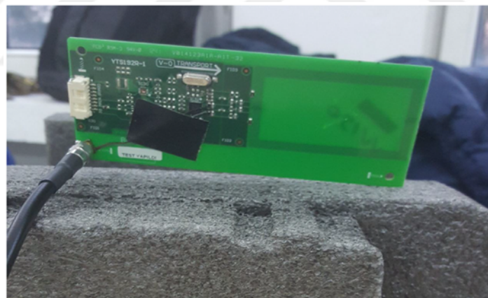
Figure 4.15. Experimental setup of reader with rectangular antenna.
