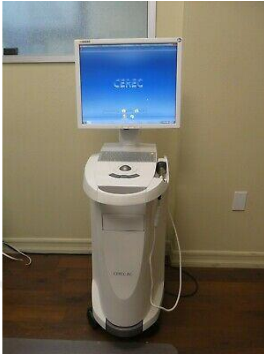
Figure 5.8: CEREC CAD\CAM intra-oral scanner
