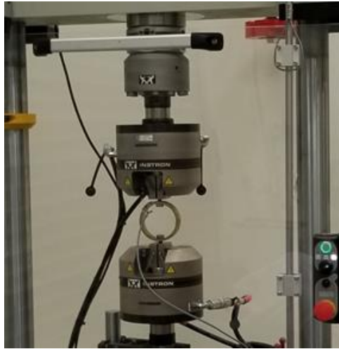
Figure 2.3. Proving ring calibration setup
