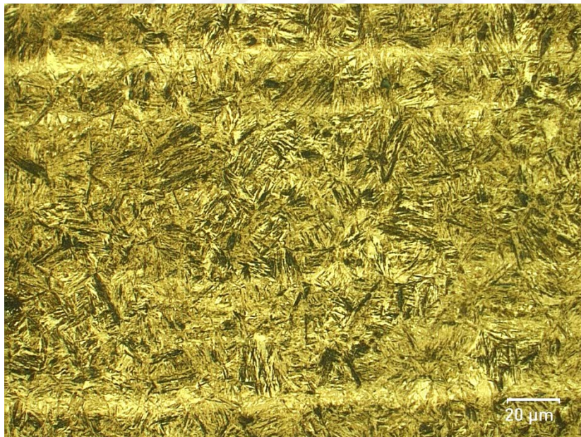
Figure 4.16. Optical micrograph of isothermally held sample at 270°C for 3 hrs.
