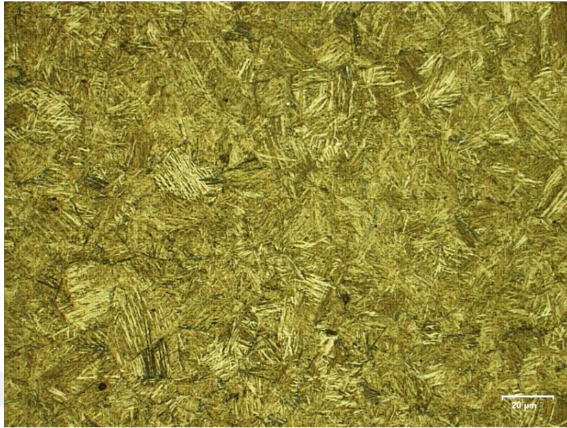
Figure 4.22. Optical micrograph of isothermally held sample at 250°C for 5,5 hrs.
