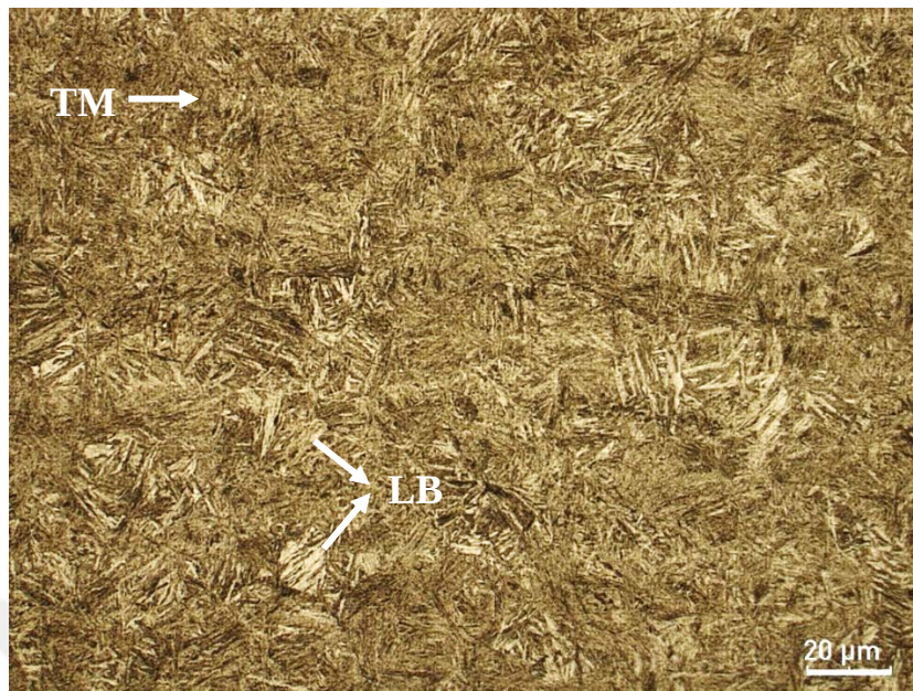
Figure 4.18. Optical micrograph of isothermally treated sample at M 50 270°C for 3 hrs
