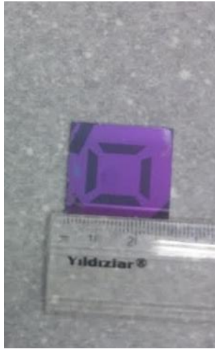
Figure 4.24. Picture of undoped and shaped Si layer on SOI wafer
