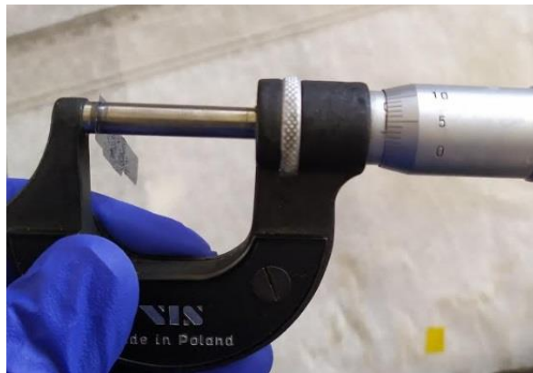
Figure 4.36. Image of measuring thickness with micrometer. Flexibility of 30\ \mu\text{m} thick silicon layer coated with SOG on kapton tape. L=10\text{mm} W=6\text{mm}
