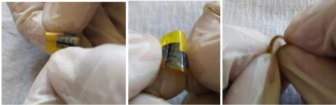
Figure 4.37. Flexibility of 30 \mu\text{m} thick silicon layer coated with SOG on kapton tape. L=10mm W=6mm
