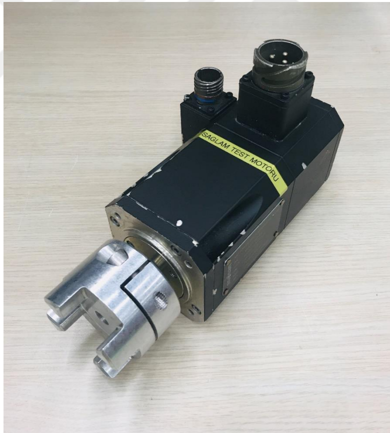
Figure 3.1. The Test Motor (400W PMSM)
