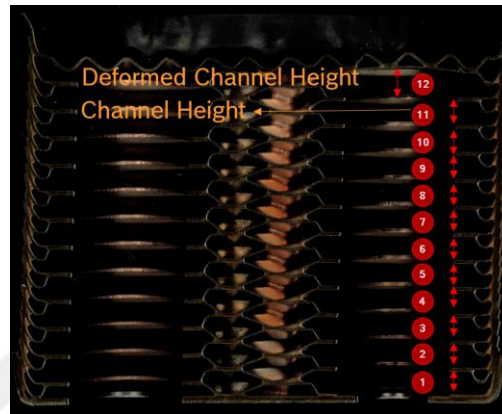
Figure 4.10. ImageJ Channel Port Measurement for AISI 316L Top Plate Used PHE Sample 1 Surface D (36 bar Max)
