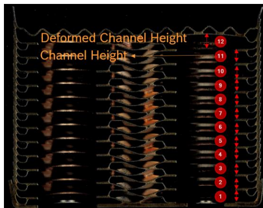
Figure 4.8. ImageJ Channel Port Measurement for AISI 316L Top Plate Used PHE Sample 1 Surface B (36 bar Max)
