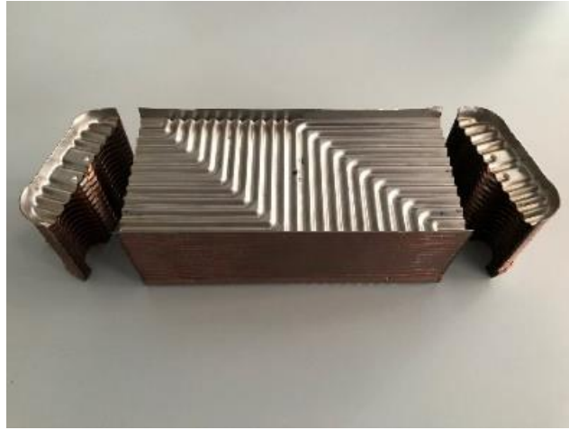
Figure 4.6. AISI 316L Top Plate Used C-PHE Cut-Out Sample
