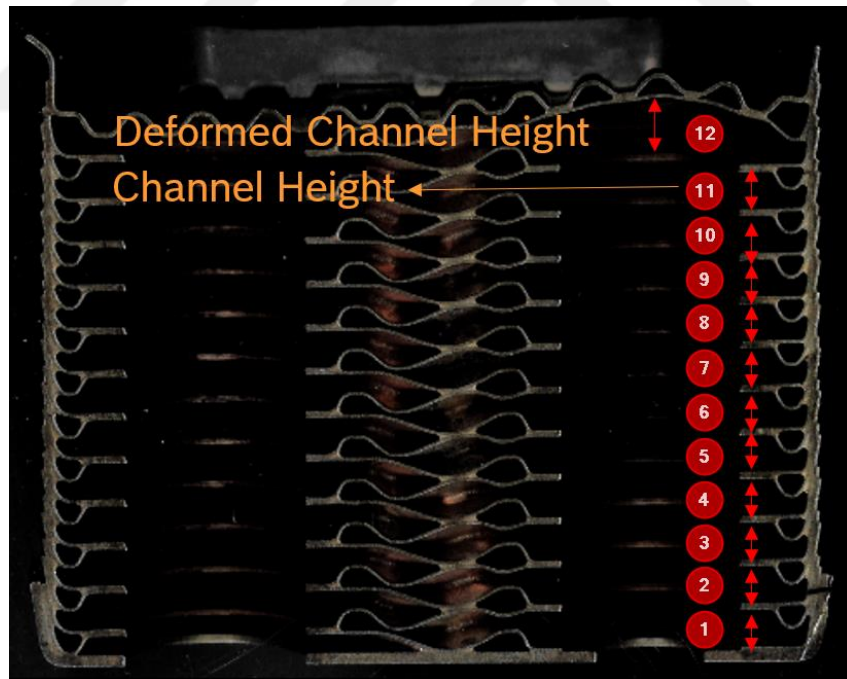
Figure 4.5. ImageJ Channel Port Measurement for AISI 304L Top Plate Used PHE Sample 1 Surface D (36 bar Max)
