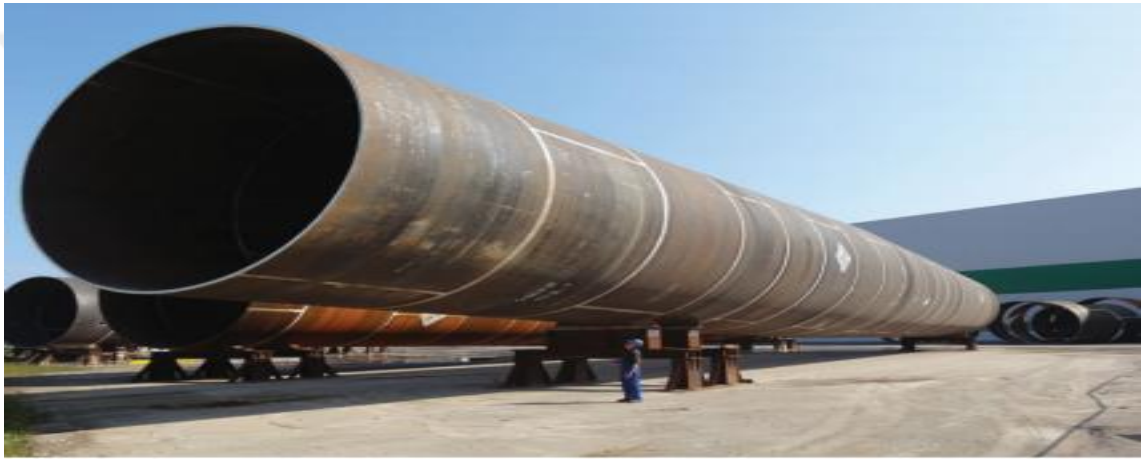
A 7.5 m diameter monopile for Gode Wind Offshore Wind Farm. DONG Energy. (Online version in colour.)
