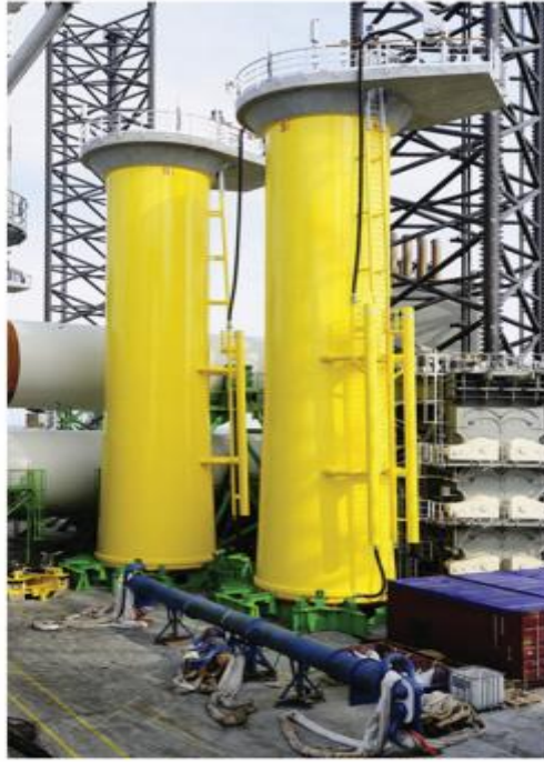
Transition piece for Borkum Riffgrund Offshore Wind Farm. DONG Energy. (Online version in colour.
