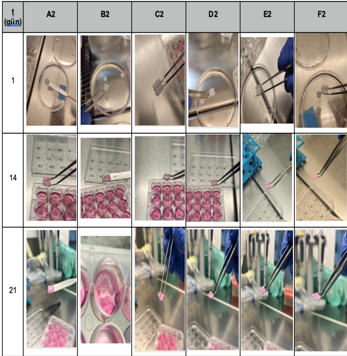
Figure 5. 13. 3D printed hydrogels produced for integrity analysis of Col/ALG (C: 0.82 mg/mL; ALG 2% w/v; MC 4% w/v).
