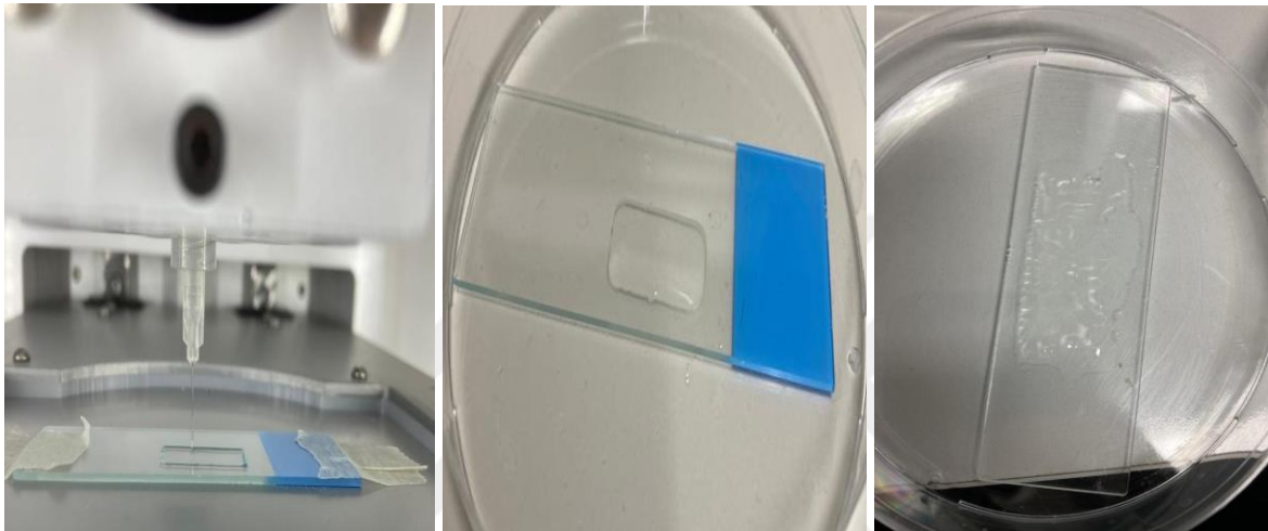
Figure 4. 2. Photographs during printing and crosslinking of C/ALG scaffolds
