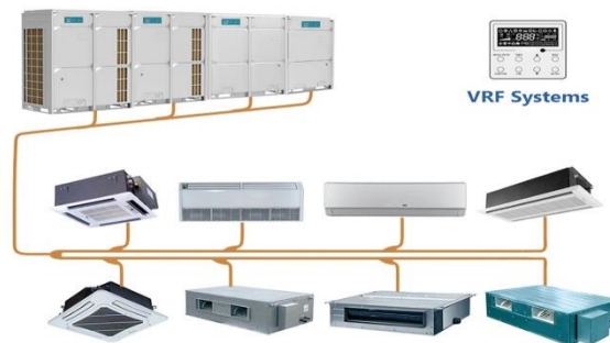
Figure 5.3. Typical VRF Heat Pump System
