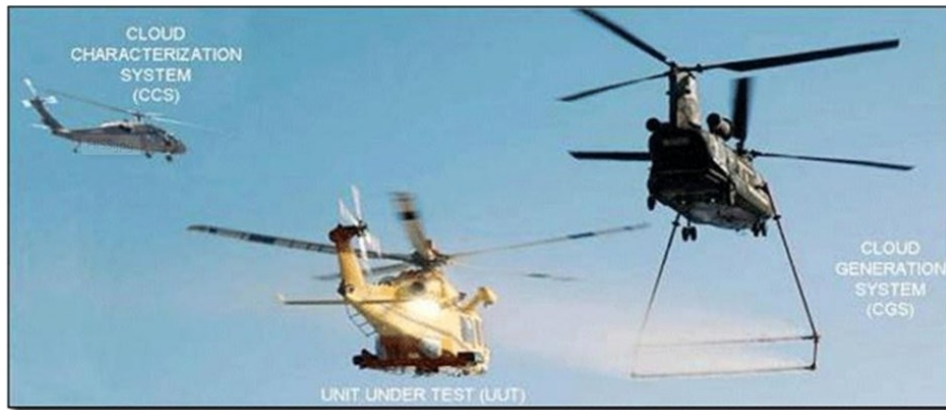
Figure 17: In-flight Icing Test [39]
