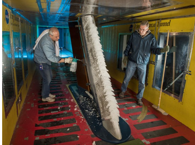
Figure 1: NASA Icing Wind Tunnel In-flight Icing Test [24]
