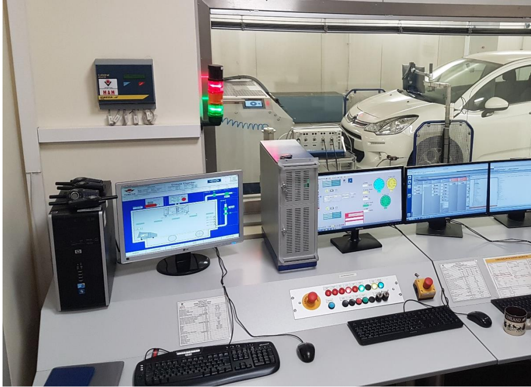
Figure 6.8 : Validation tests on chassis dynamometer.
