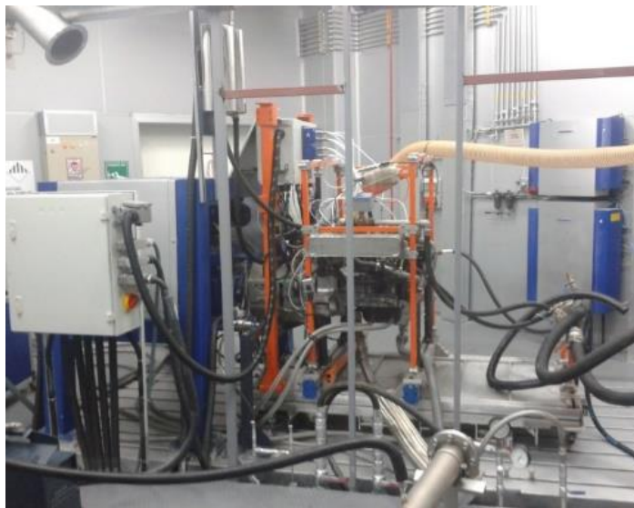
Figure 4.8 : Internal combustion engine testing at engine dynamometer.
