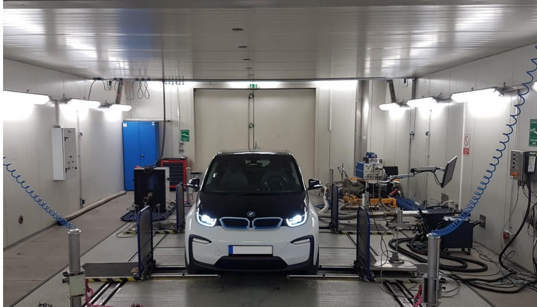
Figure 3.4 : Vehicle testing at chassis at TUBITAK dynamometer with BMW i3.
