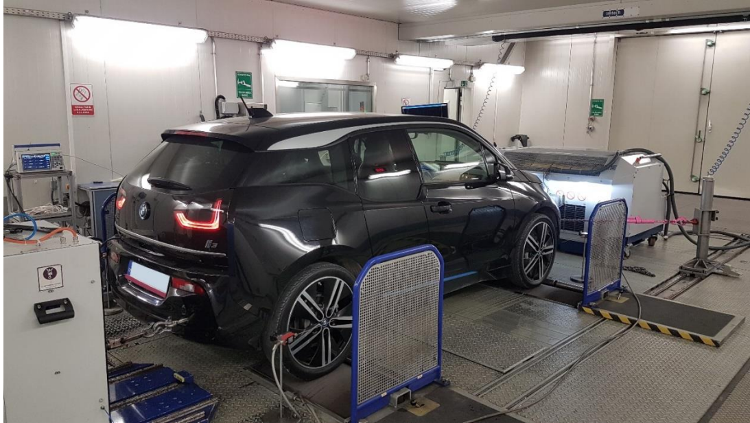
Figure 4.17 : Electric vehicle emission map model developmet tests.
