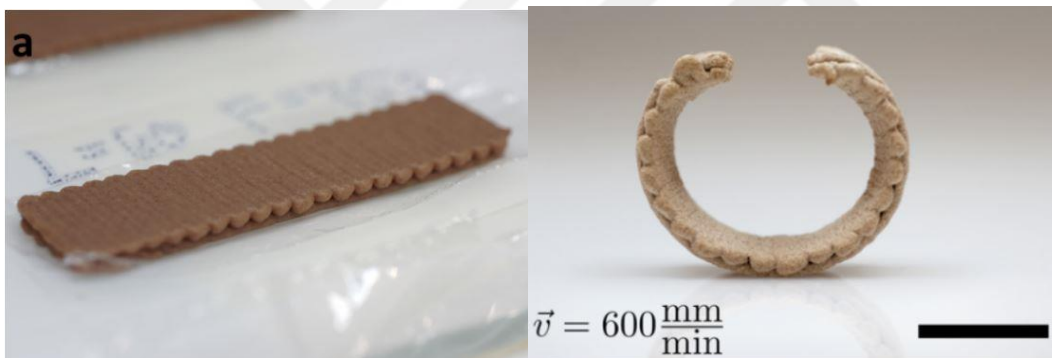
Figure 2.5. Direct Ink Writing of wood ink composed of 100% wood-based material, wood flour, and natural binders (Kam et al., 2022)
