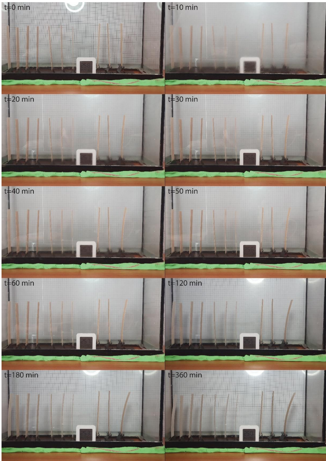
Figure 3.1. Photographs taken during the total thickness and bilayer ratio test
