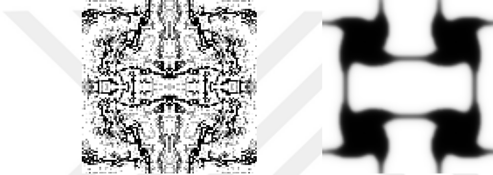
Figure 5.3: Optimum topology of a unit cell optimized without using Helmholtz filter (Left). Optimum topology of the same unit cell, optimized using Helmholtz filter (Right). Both unit cells have been optimized for negative Poisson's ratio under linear analysis, and the domain is discretized into 100x100 mesh.
