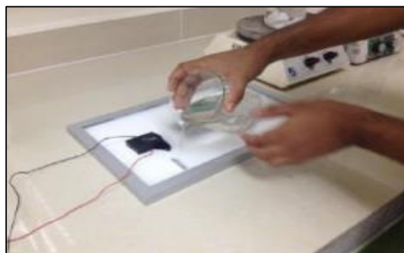
Figure 2.2: Melted PCM Pouring On The Rear Part Of PV [42].
