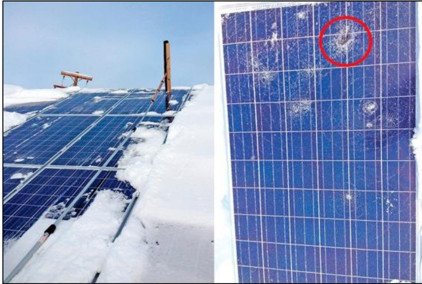
Figure 2.8: The Effect Of The Snow On The Model [89].
