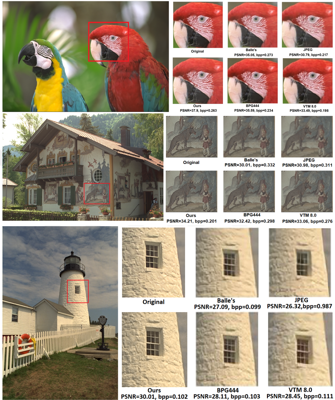
Figure 7.1: The qualitative performance comparison of the our reconstructed images with existing methods, such as Balle et al. (Ballé et al., 2016), BPG444 (Bellard, ), JPEG (Skodras et al., 2001), and VTM 8.0 (fau, ). These images are taken from KODAK(Kodak, 1993) dataset.
