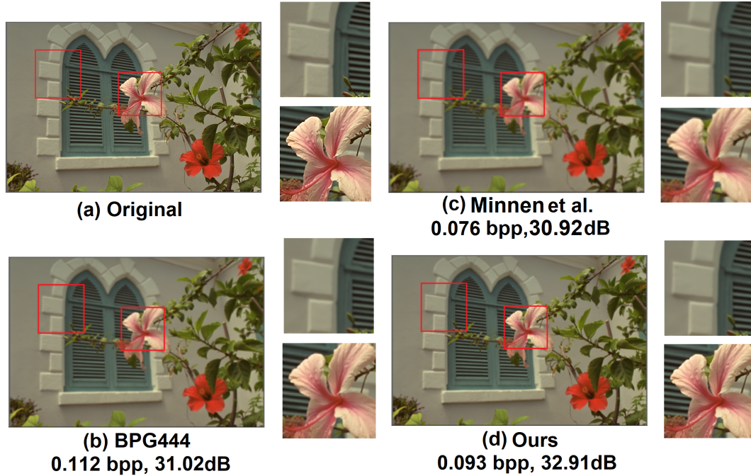
Figure 7.5: Qualitative performance. At low bit rates, visual assessment comparison with two earlier methods (Minnen et al., 2018) (Bellard, ) on KODAK dataset.
