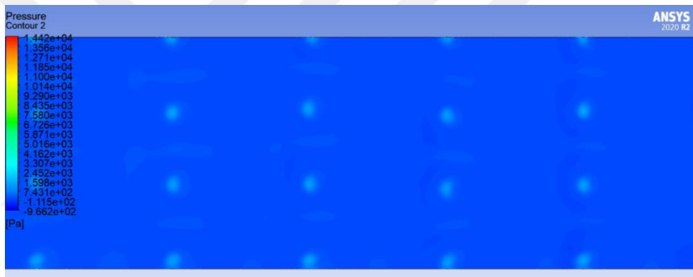
Figure 3.22. Top view of pressure distribution on the smooth absorber.
